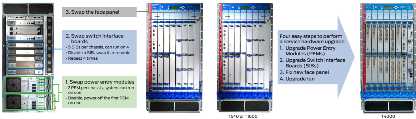
Figure 3: The in-service hardware upgrade of T640 to T1600
