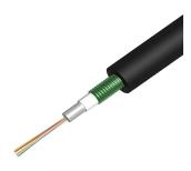
Fiber OSP cable, PE, Gel-filled Central Tube, CST, 12 fiber, Singlemode G. 652.D and G.657.A1, Meters jacket marking, Black jacket color
